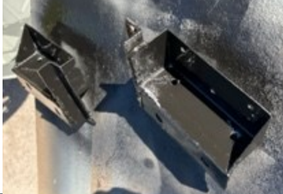
Above and adjacent: The angle iron sill edging and the front supports cleaned and new steel welded into them
