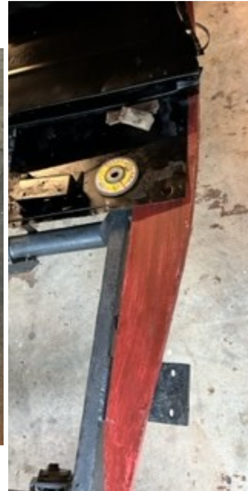
Above: The passenger side sill thickened, cut out with a band saw, painted, and angle
