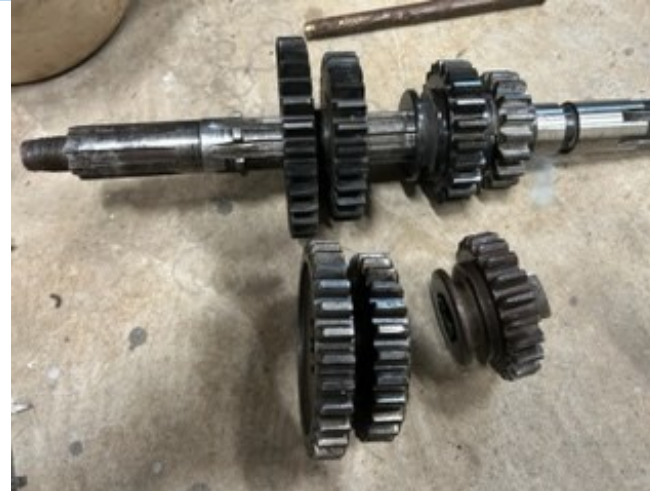
Above: The new main shaft gears are the same as the old ones
