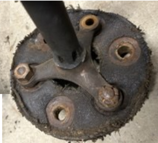
Above: One of the original flexible couplings and adjacent one that a friend made on a CNC machine.
