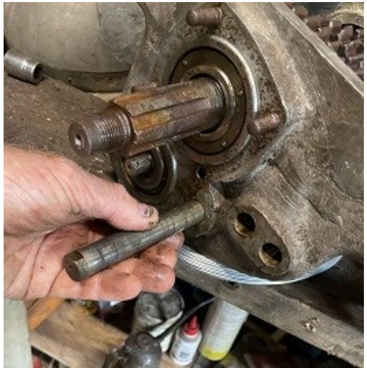
Above: The layshaft being removed
