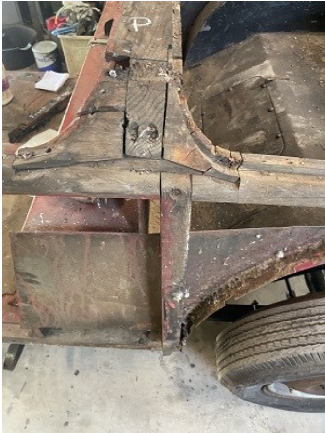
Above: The large rib timber assembly. It goes over the top of the Riley in front of the boot
