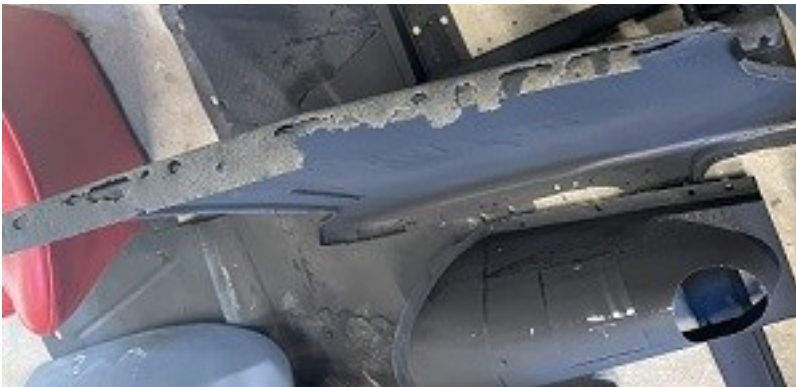
Opposite: the base of the tub after sandblasting
