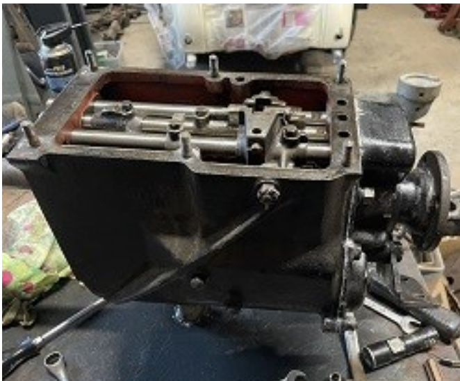
Above: a cleaned and rebuild gearbox
