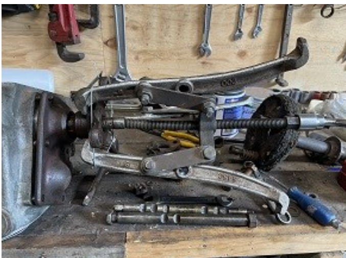
Above: The layshaft being removed
