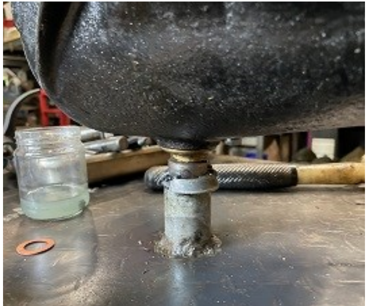
Above: The post is threaded into an RM sump plug and the tube the post fits into is welded to a plate that sits on the bench.
