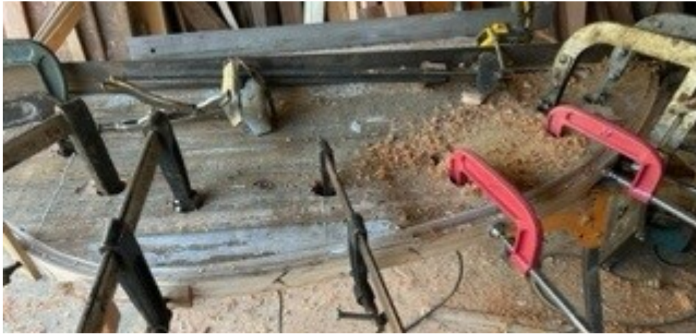
Above: Wheel arch template with strips of thin Hickory, glued and fixed into place with 'G' clamps.
