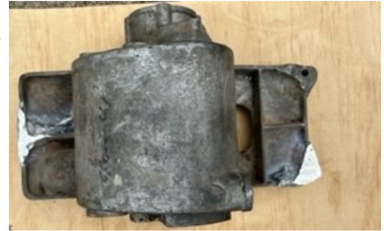
Above: The fixing points on the bottom of the box milled of swarf and rebuilt using the new gears obtained in Victoria.
