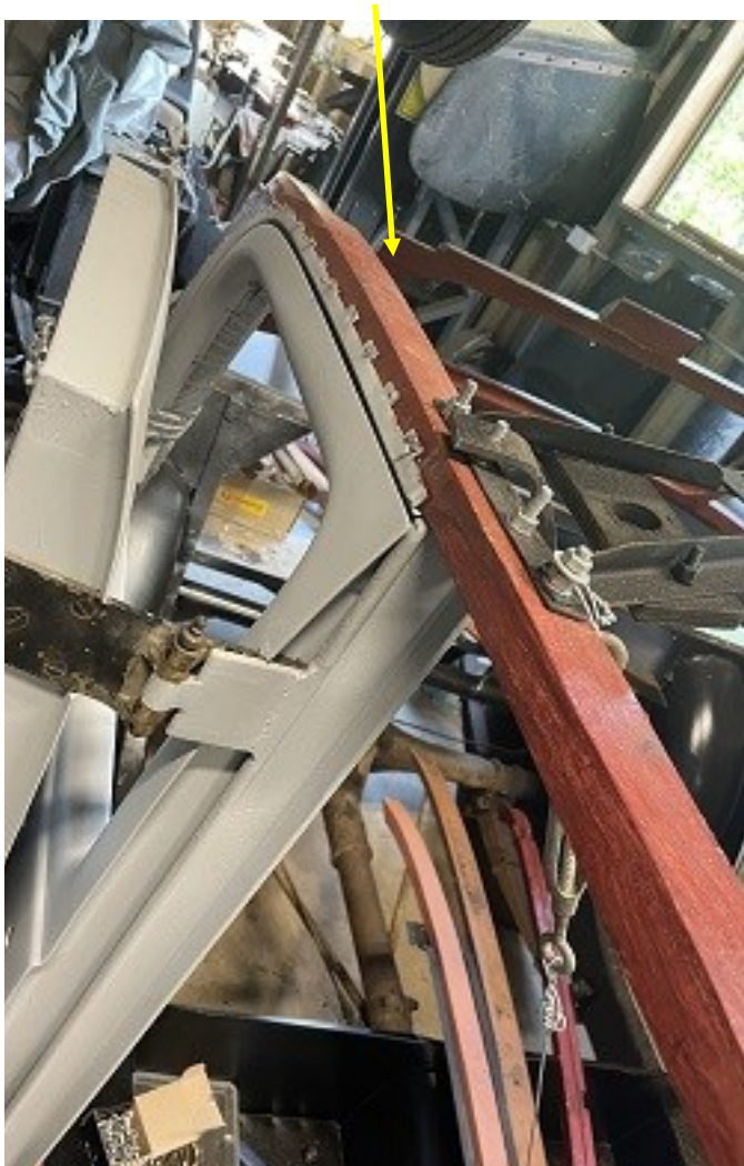
The cant rails (the pieces that go over the doors) were basically the same as on other RMs.
