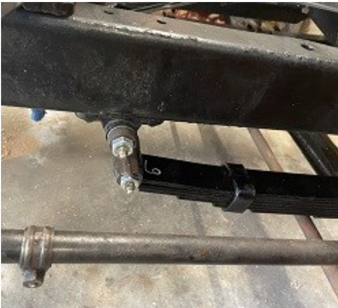
Above: without the load of the body the front shackle seems to be in the correct position at 5. 30 o'clock.
