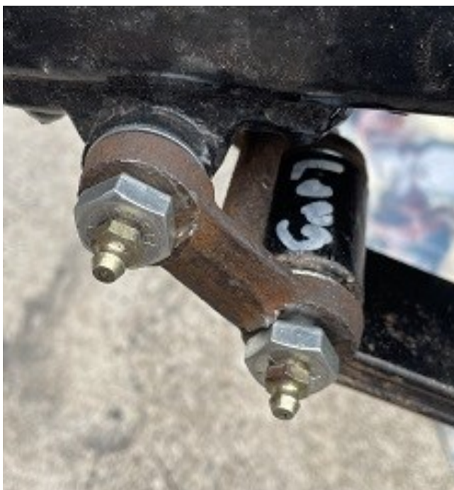
Above: The shackles too far forward and below: The rear shackle position. They are about 2.30 O'clock—too close to 3 O'clock putting them at risk of swinging in the wrong direction.
