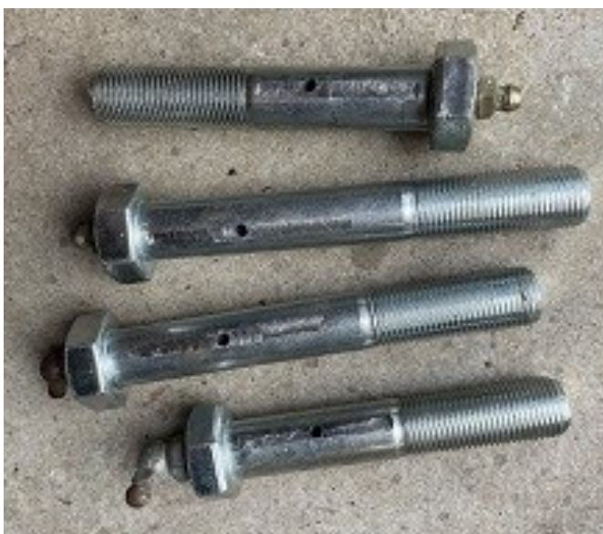
Above: The shackle pins are high tensile steel and each was purchased of a length to fit the various spring hanger requirements.
