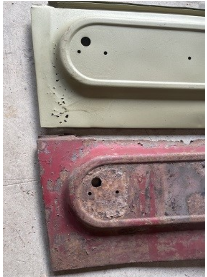
Above: Spare wheel doors ready to be grafted together
