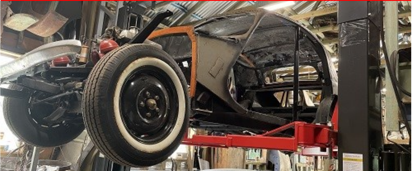
Above: The progress on the RMA restoration is apparent. The engine runs, transmission is good. The timber frame completed and the body fitted
