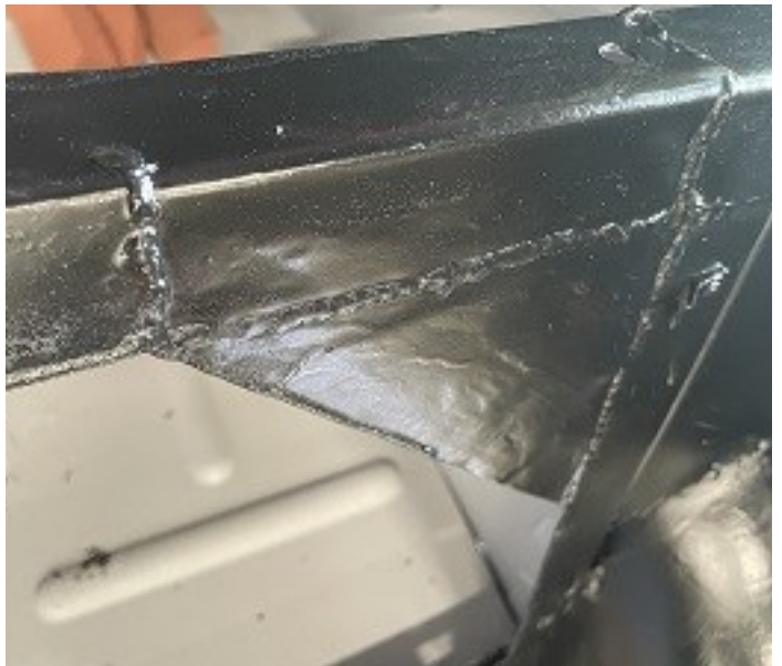
Below: pictured are other commonly found splits behind the rear passenger seat
