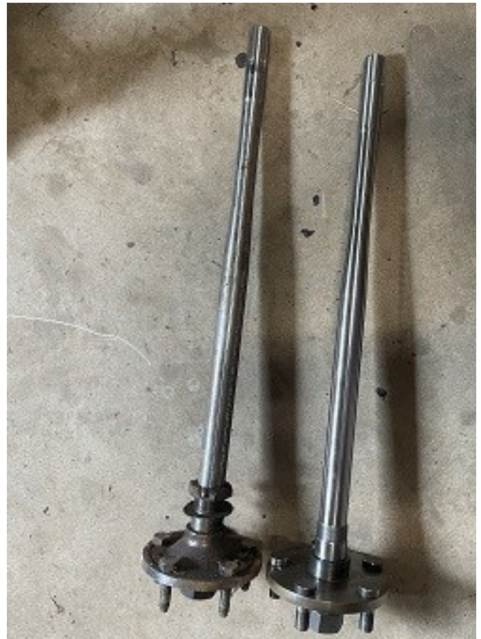
Above: On the left is an RMB half shaft and on the right is an Adelphi half shaft.
