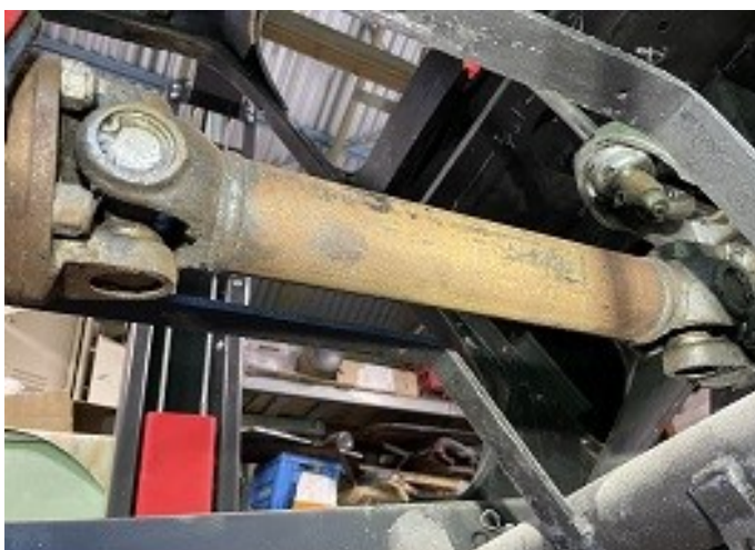
Above: Surface rust on the drive shaft and wobbly universal joints.
