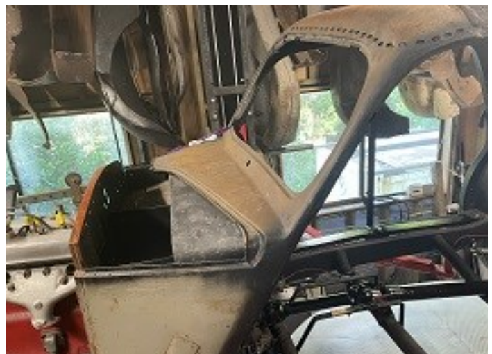
Below: Surface rust on the window surround
